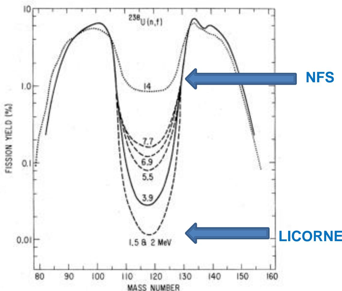
FIG. 1. Mass-yield curves for monoenergetic-neutron-induced fission of  $^{238}\text{U}$ .
