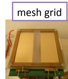
**Segmented THGEM** provides better energy resolution than mesh grid along the beam path.
