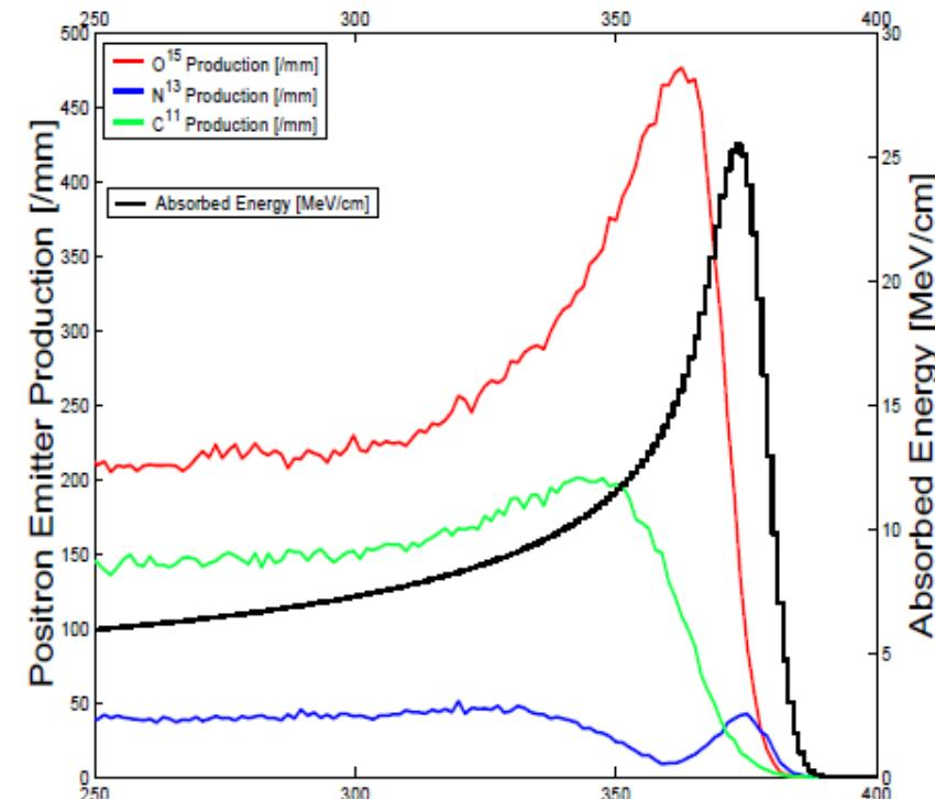
Therefore depth distribution of induced activity does not mimic the Bragg peak. The distal edge of the Bragg peak can be assessed.
