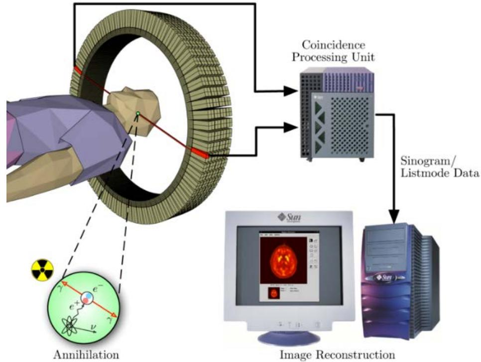
**PET tomograph is used to measure proton induced activity in tissue**
