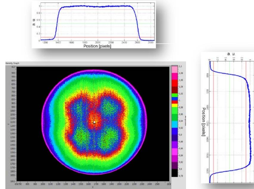
Profile of the 60 MeV proton beam from AIC-144 cyclotron
