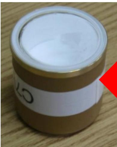
1 CLYC:Ce sample enriched with  $^7\text{Li}$  to emphasize the fast neutron detection
