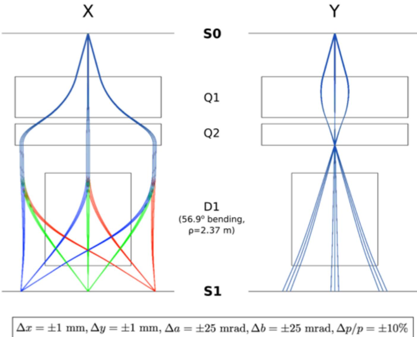
Figure 2: Results of the ion-optical calculations for the particle trajectories from S0 to S1. Left and right panels represent horizontal and vertical trajectories, respectively, for the particles with  $\Delta x = \pm 1$  mm,  $\Delta y = \pm 1$  mm,  $\Delta a = \pm 25$  mrad,  $\Delta b = \pm 25$  mrad, and  $\Delta p/p = \pm 10\%$ .
