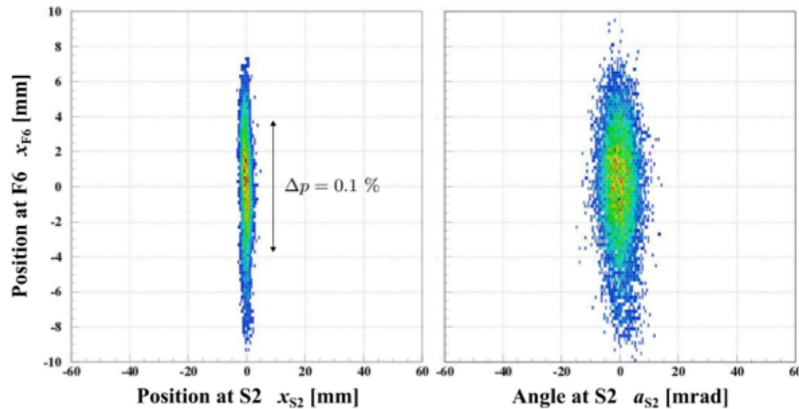
Figure 7: Correlation between  $x_{F6}$  and the position (left) and angle (right) at S2 for a  $^{16}\text{O}$  beam at 247 MeV/u. Upright correlations observed in the figures indicate that the lateral and angular dispersion-matching conditions are fulfilled.
