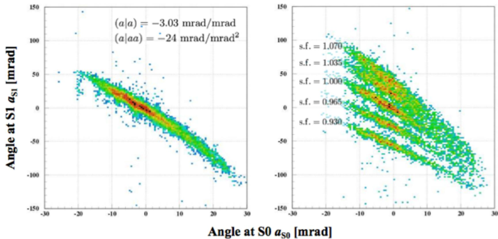
Figure 4: Correlation between the angle at the focal plane S1 and the angle at the focal plane S0 for a proton beam.
