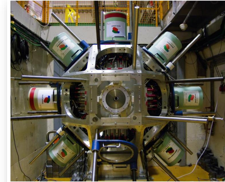
8 detectors of EXOGAM arranged into ring around the target at every 45° so angular correlation measurements could be performed
