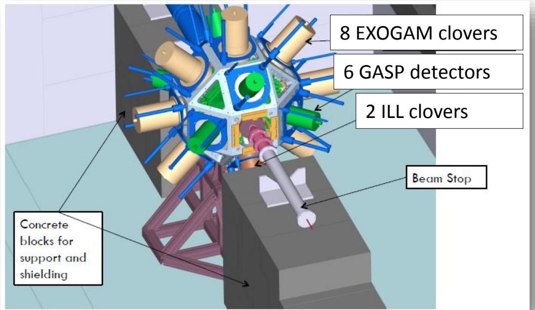
16 Ge detectors of EXILL array: 8 of EXOGAM, 6 of GASP, and 2 from ILL collaboration – coincidence measurements of gamma rays
