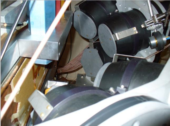
8 large volume ( $14.5 \times 17$  cm)  $\text{BaF}_2$  Scintillation detectors, were placed at back angles regarding the beam direction (theta 129 to 160 degree).
