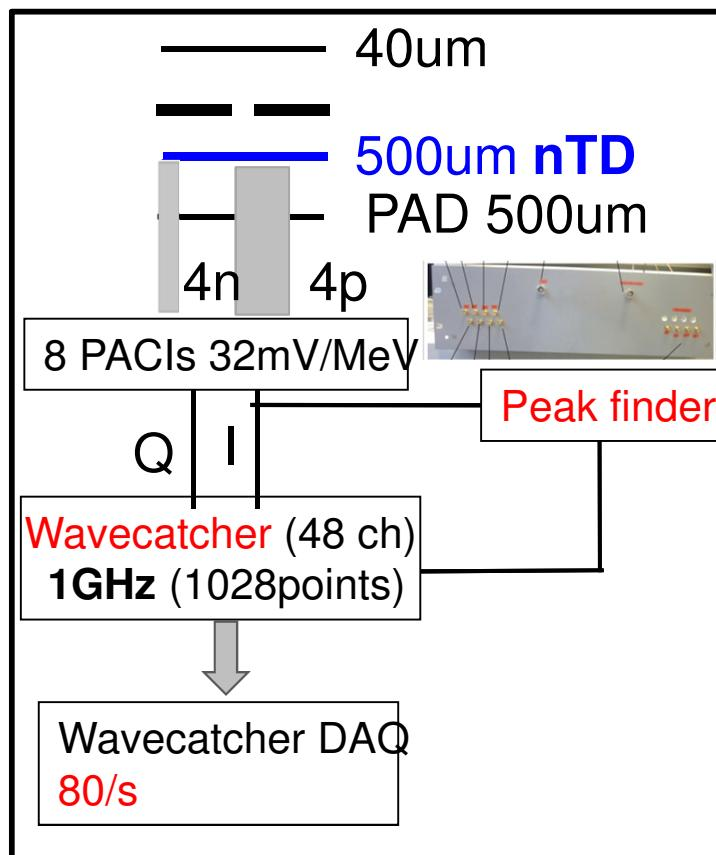
Add a  $\Delta E$  detector for PID
