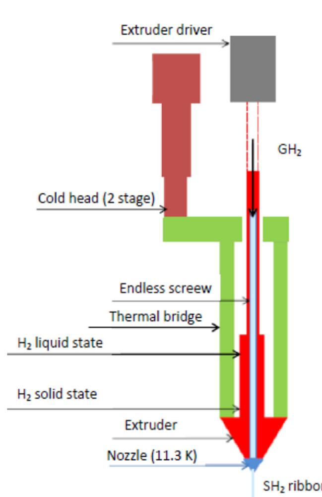
Cryogenic system in the cryostat
